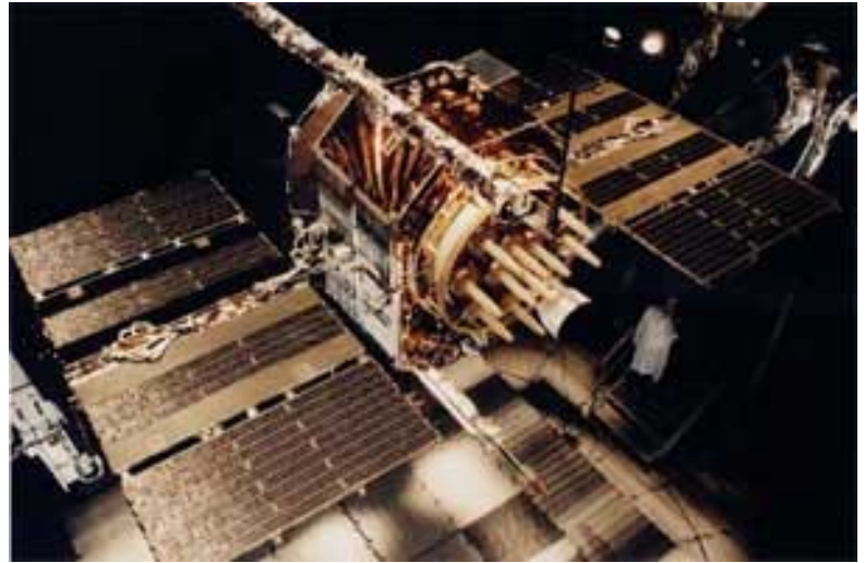
Image of a GPS satellite. Small rocket boosters on each satellite keep it flying in the correct path. The satellites have a lifetime of about 10 years until all their fuel runs out.
