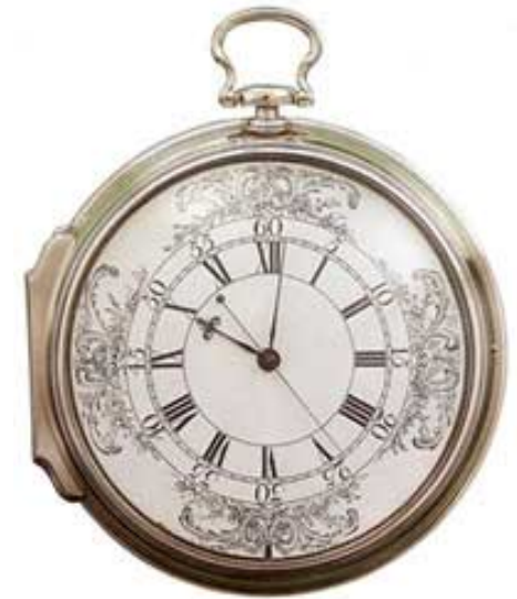
John Harrison's final masterpiece, made around 1760, was a hand held marine chronometer.
