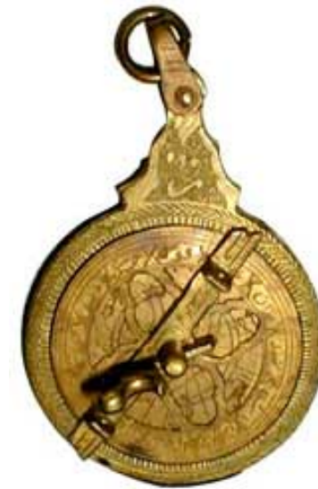
As astrolabe was used to determine the height of the sun in the sky.
